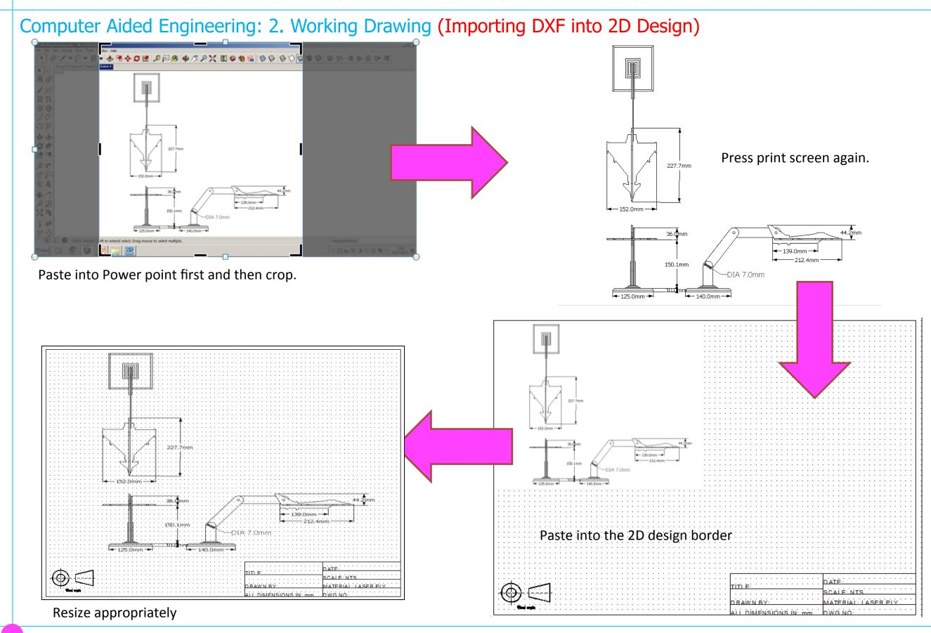
Computer Aided Engineering: 2. Working Drawing (Importing DXF into 2D Design)
